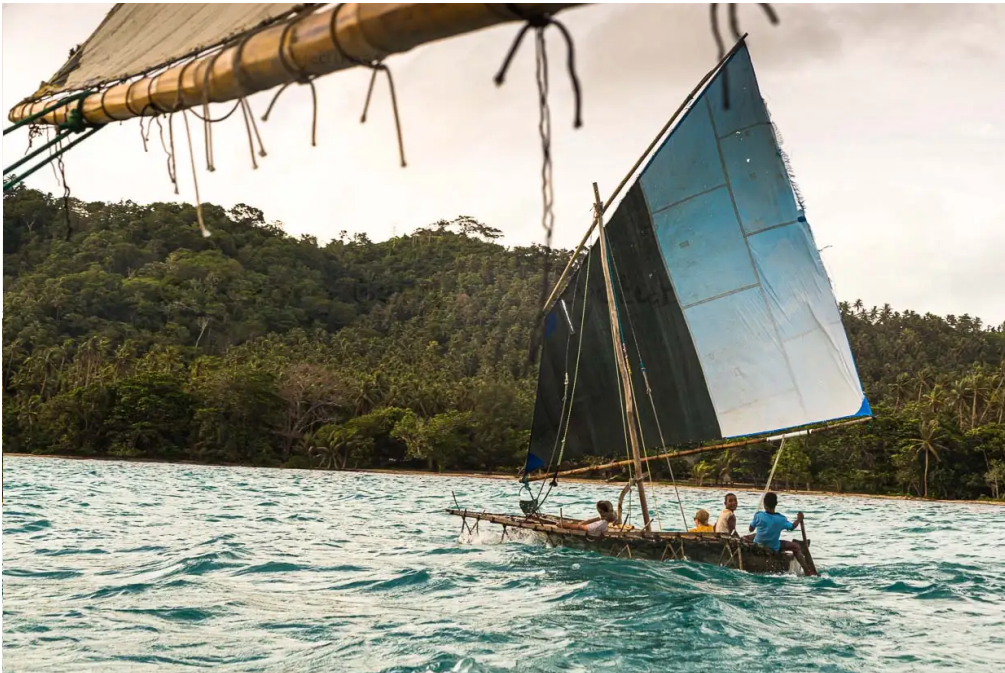
Sailing Polynesian style on a Proa (multihull outrigger sailboat) off the Deboyne Islands, Papua New Guinea. Typical of Polynesia, the Prau is an ocean-going sailing boat with delta wings and an outrigger that is always on the windward side / © Photo: Georg Berg
