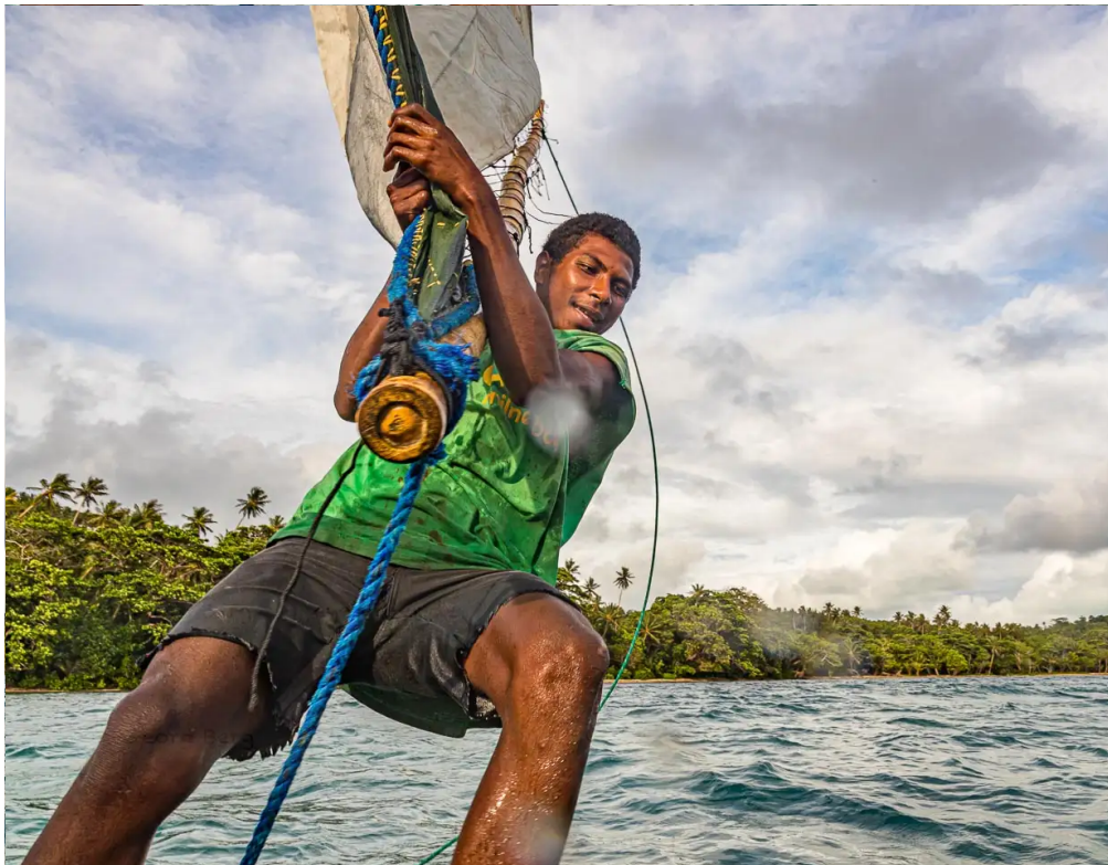
The third crew member on a Praus handles the top of the sail. Since the boat is longitudinally symmetrical, the stern and bow are exchanged when changing direction. The tip of the sail is carried around in the picture / © Photo: Georg Berg
