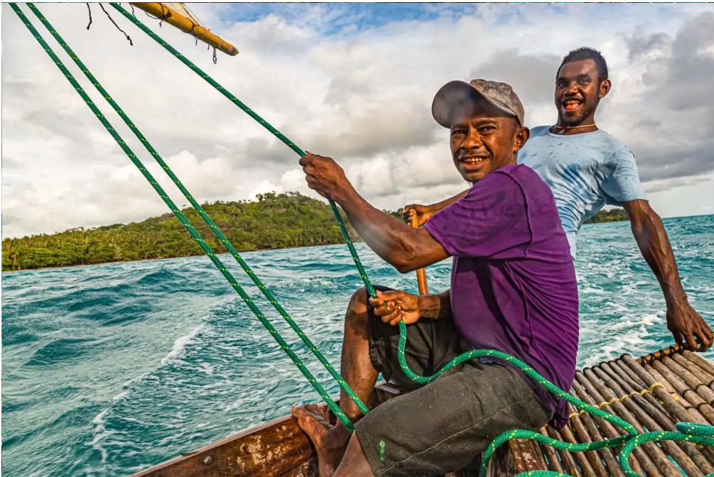
The crew of a Praus consists of at least three people. A rear determines the angle of attack of the sail. Another crew member steers by shifting weight. A loose paddle can be used to steer slightly / © Photo: Georg Berg
